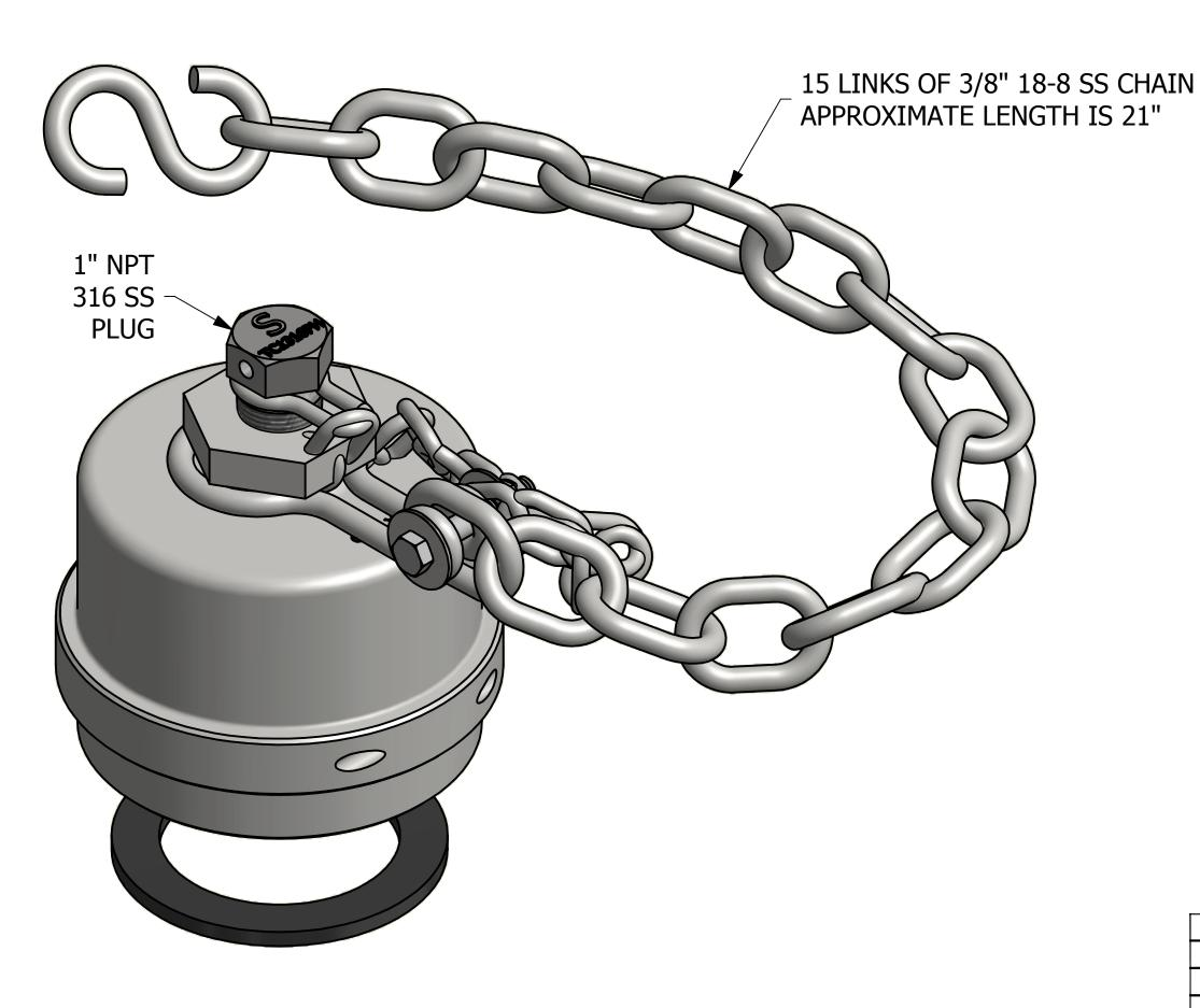
5-17-16 UPDATED TE4S416DC GEOMETRY WEB AAR# E-149523 WAS E-049013 6-18-14 REPLACED RP103MS W/ VPHC20BS RJP MCH 8-14-12 PART ADDED TO NETWORK DESCRIPTION REV BY DATE SALCO PRODUCTS, INC. QUICK CONNECT CAP 4" THREADED
